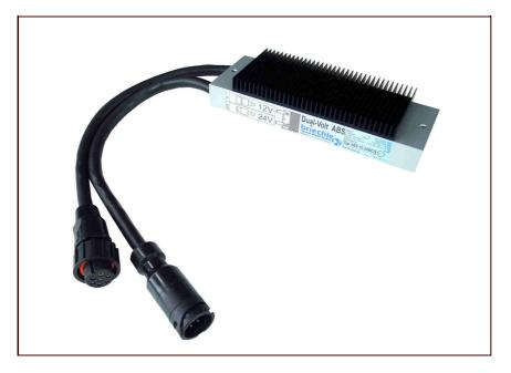
Special converter for the supply of a 24V anti lock system ABS/EBS out of 12V or 24V. The converter is equipped with ABS/EBS bayonet connectors. For inserting into the trailer cable. The contacts 6 and 7 ("CAN-Bus") are connected through. Attention! The can bus lines require a separate level shifter. Without a level shifter the brake operates correctly on the ABS level.
