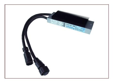
Special converter for the supply of a 24V anti lock system ABS/EBS out of 12V or 24V. The converter is equipped with ABS/EBS bayonet connectors. For inserting into the trailer cable. Male input / female output (Reverse configuration). The contacts 6 and 7 ("CAN-Bus") are connected through. Attention! The can bus lines require a separate level shifter. Without a level shifter the brake operates correctly on the ABS level.
