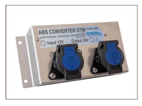
Special converter for the supply of a 24V anti lock system ABS/EBS out of 12V or 24V. The converter input isequipped with a 12V ABS/EBS socket and the output with a 24V ABS/EBS socket. The converter is mounted in a stainless steel rack and is ready for use. Preferential for trailer side mounting. Connection with the truck by the use of a 12V plugplug-cable. The 24V trailer plug will be plugged in the converter. The contacts 6 and 7 ("CAN-Bus") are unequipped.
