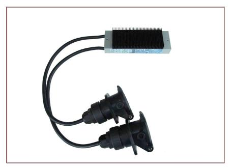
Special converter for the supply of a 24V anti lock system ABS/EBS out of 12V or 24V. The converter input is equipped with a 12V ABS/EBS socket and the output with a 24V ABS/EBS socket. Preferential for trailer side mounting. Connection with the truck by the use of a 12V plugplug-cable. The 24V trailer plug will be plugged in the converter. The contacts 6 and 7 ("CAN-Bus") are unequipped.
