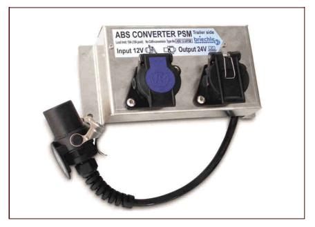
Special converter for the supply of a 24V anti lock system ABS/EBS out of 12V or 24V. The converter input is equipped with a 12V ABS/EBS socket and the output with a 24V ABS/EBS plug. The converter is mounted in a stainless steel rack with a parking socket and is ready for use. Normal case: trailer side mounting. The contacts 6 and 7 ("CANBus") are unequipped.
