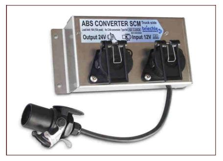
Special converter for the supply of a 24V anti lock system ABS/EBS out of 12V or 24V. The converter input is equipped with a 12V ABS/EBS plug and the output with a 24V ABS/EBS socket. The converter is mounted in a stainless steel rack with a parking socket and is ready for use. Normal case: truck side mounting. The contacts 6 and 7 ("CANBus") are unequipped.
