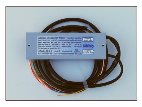
Converter to supply the lights of 12V trailers at 24V car line. Incandescent lamps and suitable RMS compatible LEDs can be operated. Please ask the LED lamp manufacturer for RMS compatibility. For further details please see our handout "LED lamps in RMS operation".
