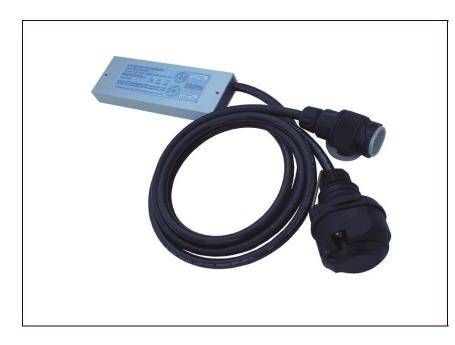
Converter to supply the lights of 12V trailers at 24V car line, including reversing lamp. Incandescent lamps and suitable RMS compatible LEDs can be operated. Please ask the LED lamp manufacturer for RMS compatibility. For further details please see our handout "LED lamps in RMS operation". Input 13 contact plug, output 13 contact socket.
