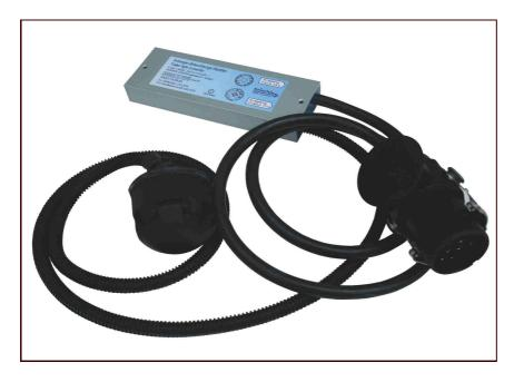
Converter to supply the lights of 12V trailers at 24V car line, including reversing lamp. Incandescent lamps and suitable RMS compatible LEDs can be operated. Please ask the LED lamp manufacturer for RMS compatibility. For further details please see our handout "LED lamps in RMS operation". Input 15 contact plug, output 13 contact socket.
