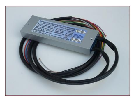
Converter to supply the lights of 12V trailers at 24V car line, including reversing lamp. Incandescent lamps and suitable RMS compatible LEDs can be operated. Please ask the LED lamp manufacturer for RMS compatibility. For further details please see our handout "LED lamps in RMS operation".
