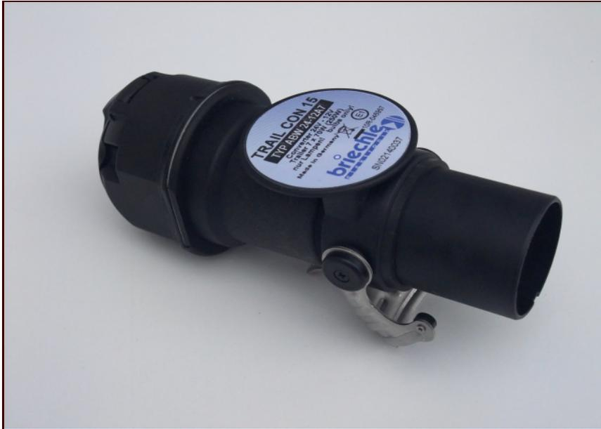
Converter to supply a 12V trailer from a 24V vehicle system as short adapter 15 pin to 13 pin, including reversing lamp. Incandescent lamps and suitable RMS compatible LEDs can be operated. Please ask the LED lamp manufacturer for RMS compatibility. For further details please see our handout "LED lamps in RMS operation".
