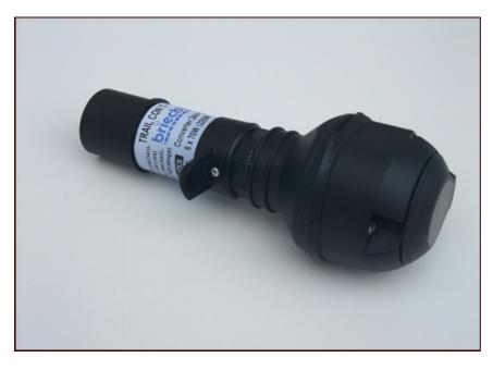
Converter to supply a 12V trailer from a 24V vehicle system as short adapter 7 pin to 13 pin, the reversing lights are not connected. Incandescent lamps and suitable RMS compatible LEDs can be operated. Please ask the LED lamp manufacturer for RMS compatibility. For further details please see our handout "LED lamps in RMS operation".
