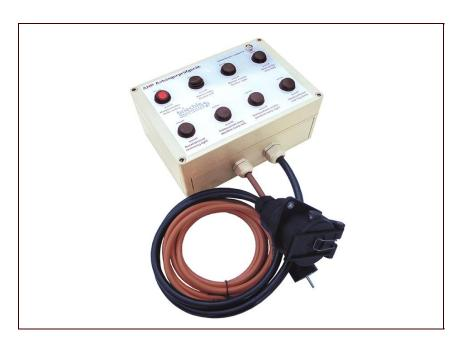
The AHP24 (trailer-test-device) is designed for testing the lighting of a trailer. The test allows to switch on and off indicator left, indicator right (integrated indicator relay), stop light, rear light left, rear light right, fog lamp and reversing light independently of each other.
