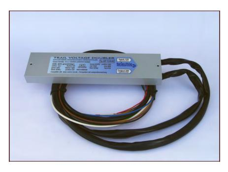
Converter for the supply of a 24V trailer from a 12V or a 24V vehicle line, high-performance, also for LEDs. For Mercedes Sprinter and Volkswagen Crafter the adaption module EC-ASV1 is required. Important: In case of high loads and long cables on the input side the current consumption could increase enormously determined by the system. Please contact us, we provide planning aid and adaption solutions.
