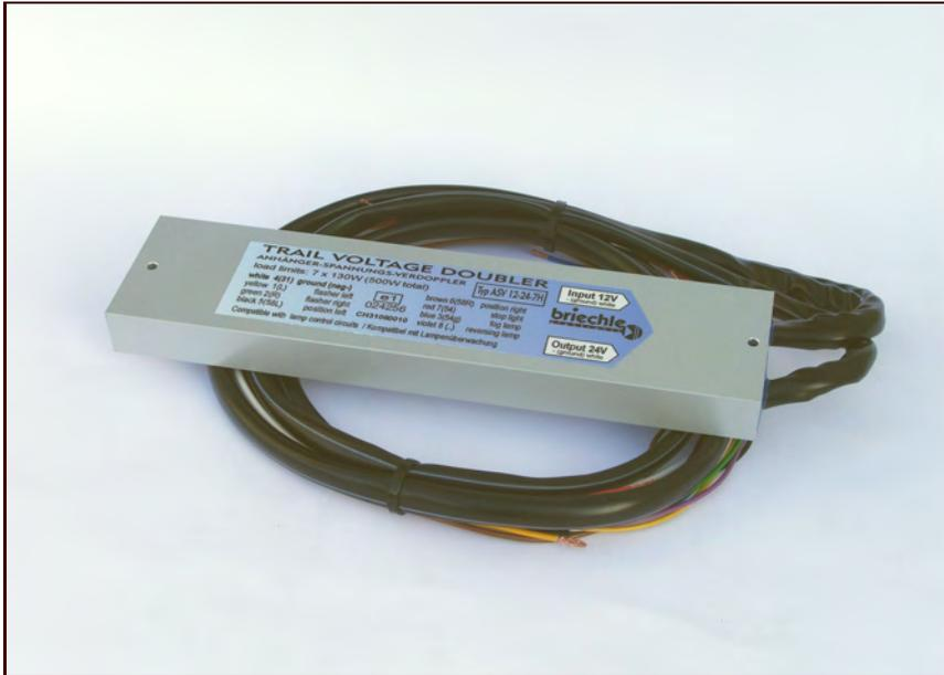
Converter for the supply of 24V trailers from a 12V or a 24V vehicle line, with reversing lamp, high-performance, also for LEDs. For Mercedes Sprinter and Volkswagen Crafter the adaption module EC-ASV1 is required. Important: In case of high loads and long cables on the input side the current consumption could increase enormously determined by the system. Please contact us, we provide planning aid and adaption solutions.
