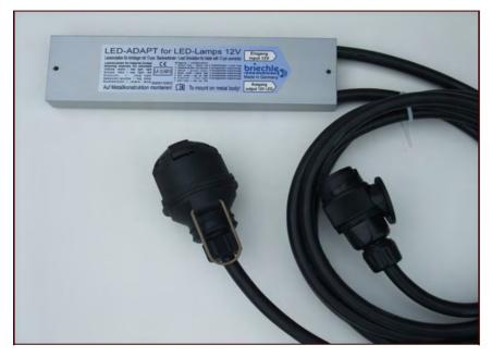
12 Volt resistor replacement load for the adaptation of light emitting diode (LED) trailer lamps at vehicles with incandescent lamp monitoring. The direction indicator lamps and the contacts 9 to 13 are looped. LED-ADAPT must be mounted on a metal surface. Important: The direction indicators must be incandescent lamps or LEDs with own monitoring. Other lines may have additional load of 10W maximum, in this case monitoring is disabled.
