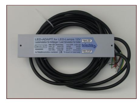
12 Volt resistor replacement load for the adaptation of light emitting diode (LED) trailer lamps at vehicles with incandescent lamp monitoring. The failure of a LED unit is indicated and the replacement load is turned off. LED-ADAPT must be mounted on a metal surface. \*\*\*CAUTION\*\*\* The connection of any bulb on the output is prohibited. The over current protection may cut off not until after several minutes!
