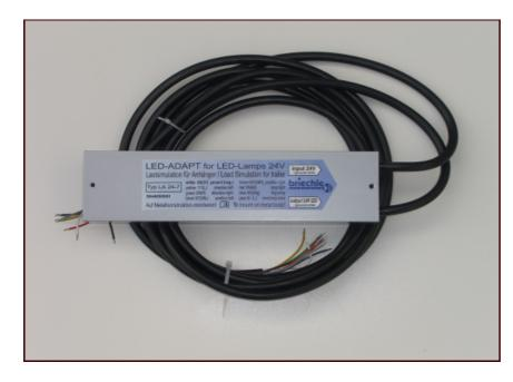
24 Volt resistor replacement load for the adaptation of light emitting diode (LED) trailer lamps at vehicles with incandescent lamp monitoring. The failure of a LED unit is indicated and the replacement load is turned off. LED-ADAPT must be mounted on a metal surface. \*\*\*CAUTION\*\*\* The connection of any bulb on the output is prohibited. The over current protection may cut off not until after several minutes!
