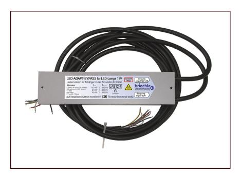
12 Volt resistor replacement load for the adaptation of light emitting diode (LED) trailer lamps at vehicles with incandescent lamp monitoring. The failure of a LED unit is indicated and the replacement load is turned off. To cool the system a metal surface is needed. The Bypass-function enables subsequent mounting of bulbs up to 95W.
