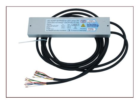
24 Volt resistor replacement load for the adaptation of light emitting diode (LED) trailer lamps at vehicles with incandescent lamp monitoring. The failure of a LED unit is indicated and the replacement load is turned off. To cool the system a metal surface is needed. The Bypass-function enables subsequent mounting of bulbs up to 180W.
