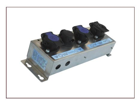
Complete Trailer unit 12V to 24V for agricultural and forestry vehicles, for lights and ABS. At the input and the output sockets are mounted. The connection to the towing vehicle and the trailer is made by intermediate cables. The converters inside are ABS 12-24 and ASV 12-24-6H and are mounted in a stainless steel metal rack together with the sockets.
