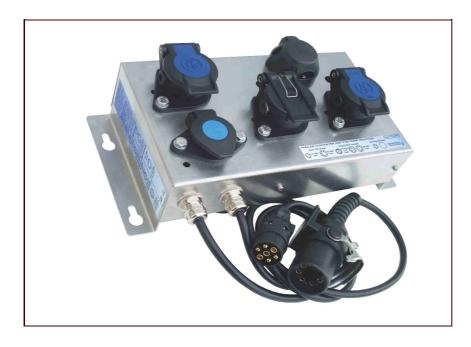
Complete Trailer unit for farming tractors 12V to 24V for lights and ABS. At the input are plugs and at the outlet are sockets. Park sockets are available when the converter is not in use to take the free plugs. The unit is mounted in a stainless steel metal rack. The converters inside are ABS 12-24 and ASV 12-24-6H.
