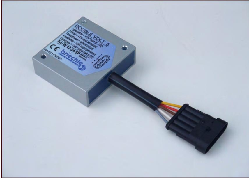
Step up voltage converter with medium power from 12V until 24V (wide range) to 24V car line. For the simultaneous supply of permanent positive and ignition positive. The total current can be shared in any relation between the both outputs.
