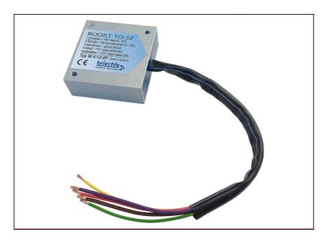
Step up voltage converter with medium power from 6V until 12V (wide range) to 12V car line. For the simultaneous supply of permanent positive and ignition positive. The total current can be shared in any relation between the both outputs.
